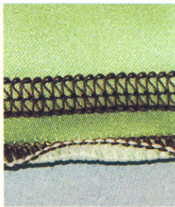
Seven-thread reverse wave stitch
